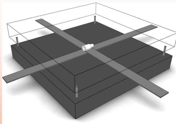
Field tests involved placement of artificial hibernacula, in this case, cement tile “sandwiches” with one tile flush with the soil surface and an upper one forming a roof (see diagram to left). Each setup had two wooden stakes laid perpendicular to each other with a rubber septum placed at the junction. Treatment setups consisted of the septum treated with IBMP and the sticks with lady beetle foot extracts.
